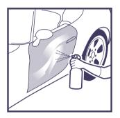
Ensure the surface is oil free and completely dry. Use  $\mathbf{Q^2M}$  PREP before applying the coating (isopropyl alcohol does not fully degrease the surface).
