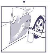
Ensure the surface is oil free and completely dry. Use **Q<sup>2</sup>M PREP** before applying the coating (isopropyl alcohol does not fully degrease the surface).
