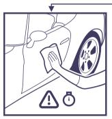
Wipe off immediately (10 – 30 seconds) after applying on the whole panel/section. Wipe off carefully, do not leave any streaks or smudges. Please note that the drying time may vary depending on a country's climate (ask your supplier for advice).
