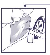
Ensure the surface is oil free and completely dry. Use **Q<sup>2</sup>M PREP** before applying the coating (isopropyl alcohol does not fully degrease the surface).
