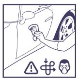
Split larger panels (roof, bonnet, SUV doors) into sections, apply carefully.
