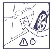
Wipe off immediately (10 – 30 seconds) after applying on the whole panel/section. Wipe off carefully, do not leave any streaks or smudges. Please note that the drying time may vary depending on a country's climate (ask your supplier for advice).
