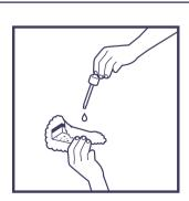
Apply a thick layer of **Q<sup>2</sup> BASE** in a criss cross motion. Pay attention to the leveling of the coating. If needed, do a second criss-cross application to achieve a perfectly even layer.
