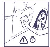
Wipe off **Q<sup>2</sup> FLEXI** shortly after application to a panel has been completed. **Q<sup>2</sup> FLEXI** is thick and requires a precise wipe off.
