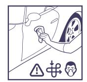
Apply  $\mathbf{Q^2}$  **FLEXI** in a criss-cross motion, ensuring full coverage of the coated panel.
