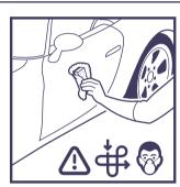
Split larger panels (roof, bonnet, SUV doors) into sections, apply carefully.
