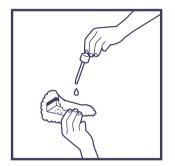
Apply a thick layer of  $\mathbf{Q}^2$  BASE in a criss-cross motion. Pay attention to the leveling of the coating. If needed, do a second criss cross application to achieve a perfectly even layer.
