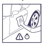
Wipe off immediately (10 – 30 seconds) after applying on the whole panel/section. Wipe off carefully, do not leave any streaks or smudges. Please note that the drying time may vary depending on a country's climate (ask your supplier for advice).
