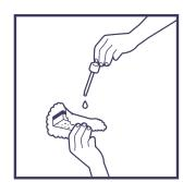
Apply the **Q<sup>2</sup> FLEXI** top coat not longer than 1 hour after **Q<sup>2</sup> BASE** has been applied to the entire vehicle.
